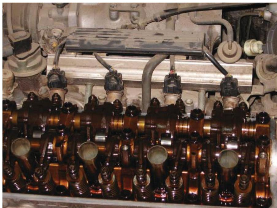
Figure 8 | Oxidation residue. (Figure courtesy of Honda.)
