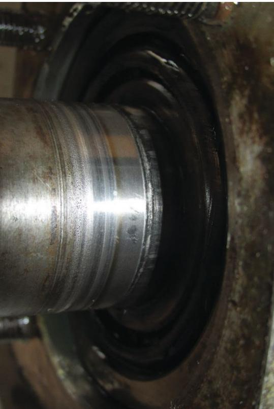
Figure 7 | Seal abrasion.
